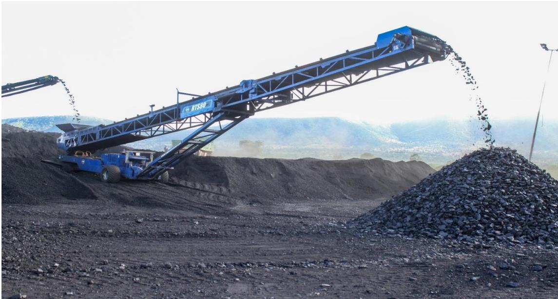
Coal processing stacker conveyor belt
